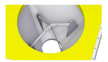
The knife cross is removable and can easily be adjusted to increase or decrease the cutting of the bag.
